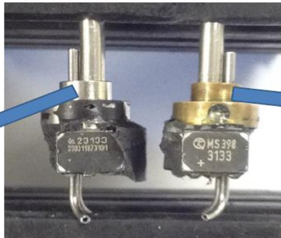
ER10C New design, #2972 Gap, no glue, the white jammed thing is putty
